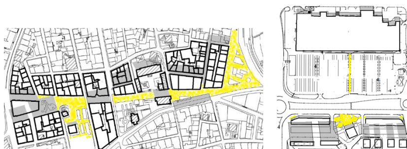
Figure 9: Shadows of buildings (20 January-11.00 a.m.) and pedestrian areas (It was prepared by calculating the shadow lengths relative to the sun's orbit at 37.87^\circ latitude)
