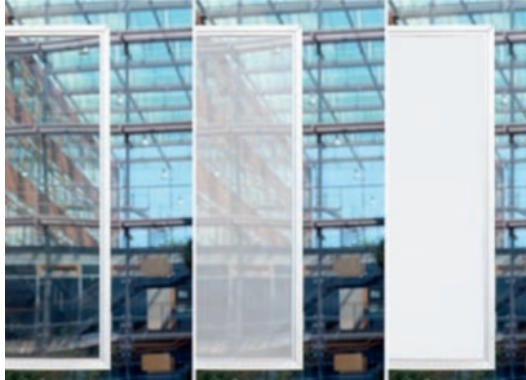
Figure 2. Thermochromic glass in different states (Ritter, 2007)
