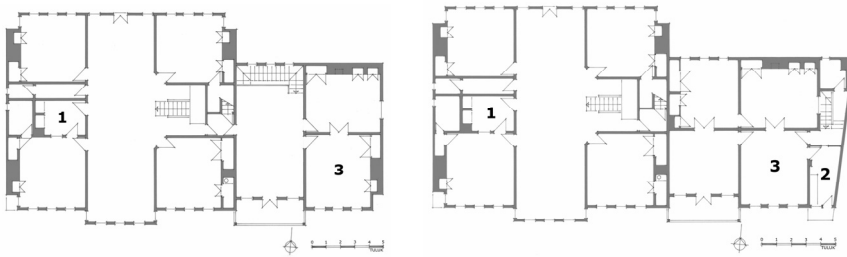
Figure 7. The second floors of the Yalçınlar Mansion (first phase restitution and existing plans)
