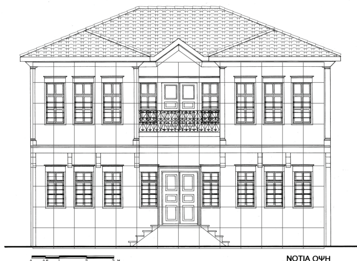
Figure 5. Façade of Chatzitzotzas Mansion in Florina. The upper floor height is 4 arşin and the ground floor height is 3,5 arşin
