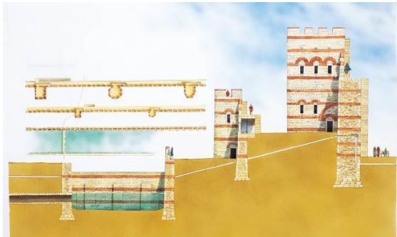
Figure 12. The Plan and the Section of the Theodosian Land Walls (Turnbull, 2004, 11)
