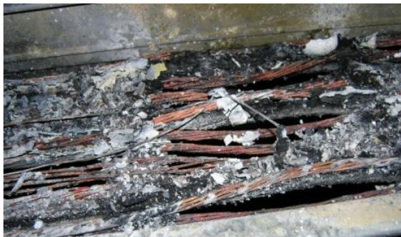
Figure 8. Damaged Electrical Cables after Fire
